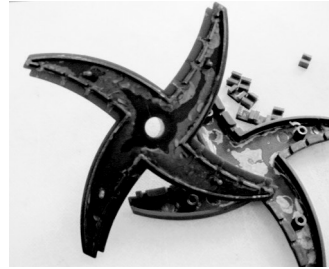
The sprinkler head separates for periodic maintenance. Film and gel from the seed jackets can clog the tiny water outlets.
